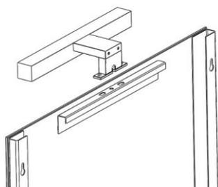
Pass the cable through the bracket and screw lighting
